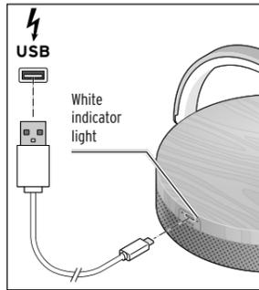
2. Plug one end of the USB-C charging cable into the connection socket on the speaker and the other end into the USB mains adapter.
