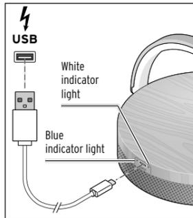
1. Plug one end of the USB-C charging cable into the connection socket on the speaker and the other end into the USB mains adapter.
